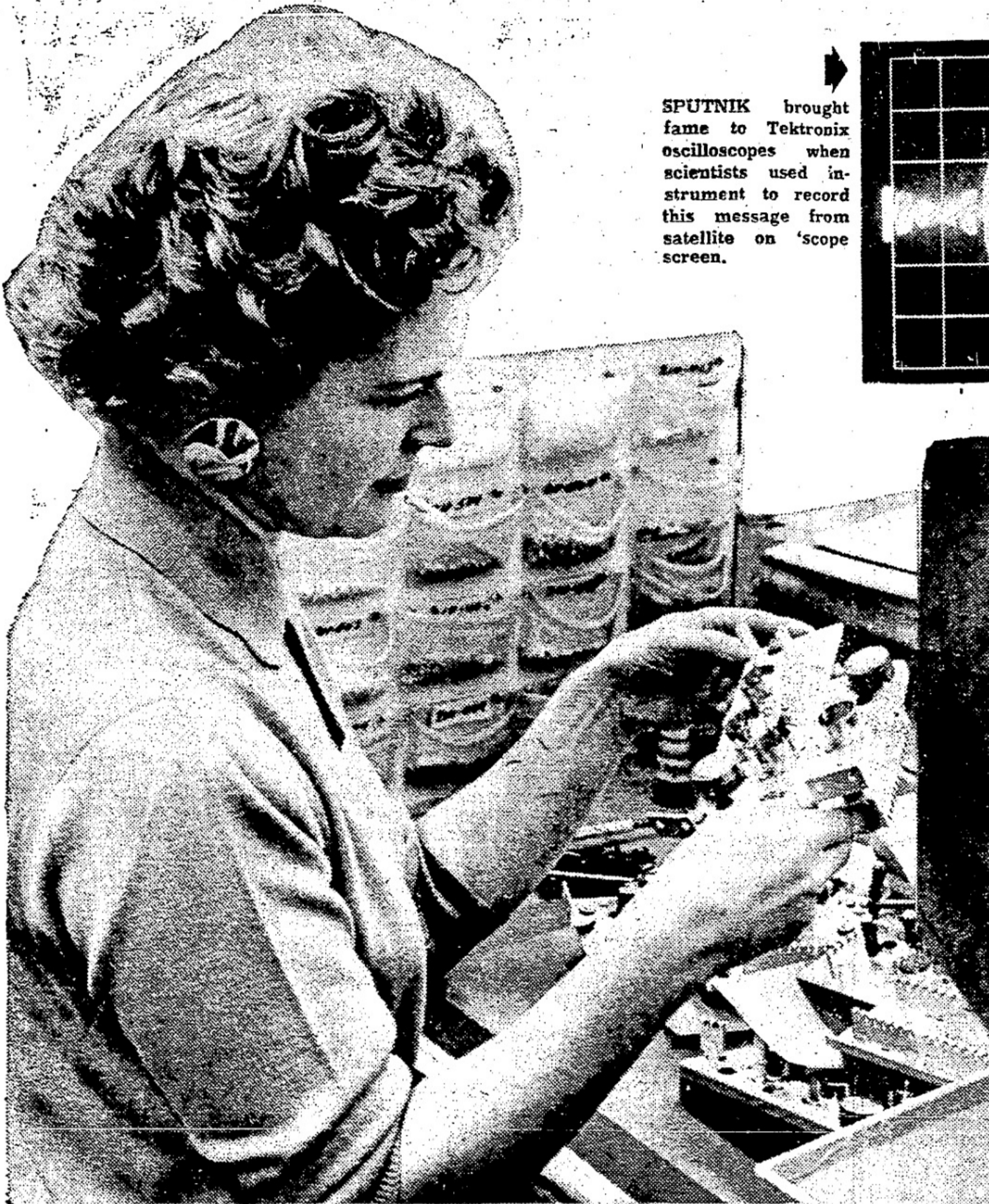
WORKING FROM chassis stamped and drilled by Tektronix presses, this assembly worker carefully places insulators in small oscilloscope. Low employee turnover, careful selection of workers and good working conditions contribute to exceptionally low rate of failures.
