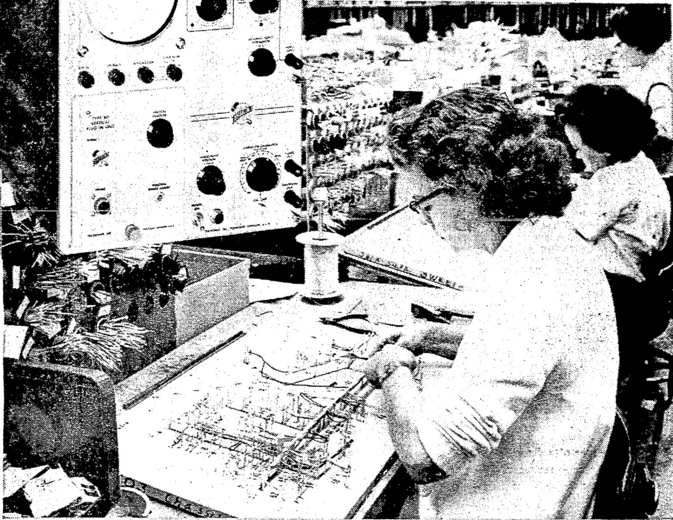
CIRCUITS, LAID out on pattern board in full colors, are followed by this assembly worker who fastens complete pattern together as another step in assembly-manufacture of oscilloscopes. Jobs like these provide work for some 3,000 Oregonians as well as an additional 600 in other out-of-state Tektronix offices and plants. Finished 'scope of $40-million-a-year business is in center.
