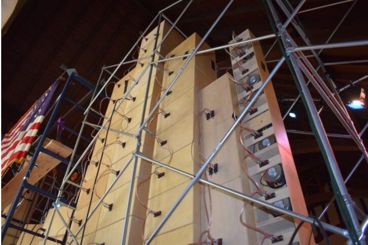
The rear of the Wall of Sound has been as meticulously recreated as the front; like the original, only the speakers replicating Jerry Garcia's guitar column are open-backed.
