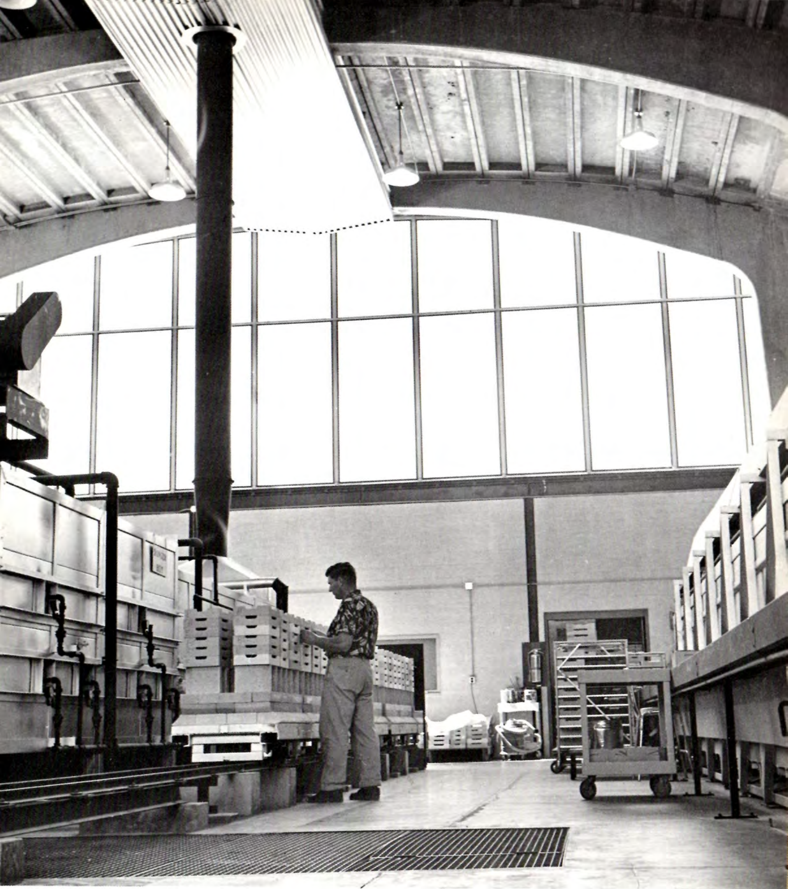
CERAMIC PRODUCTION —The kiln section of the ceramic manufacturing plant is shown here. Ceramic production includes the unique ceramic terminal strips used in Tektronix instruments and such specialized items as isolation shields, bushings, and mounts for cathode-ray tubes, and attenuator, probe, and capacitor parts.
