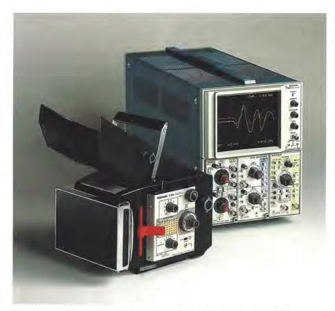
The 5116 color display can easily be photographed in color by either a Tek C5C or Tek C59A camera pack. Each has special attributes depending on the film chosen.
