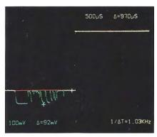
A particular advantage of color is in difficult-to-see signal deviations. In this example, one color is used for the reference trace and the color shows the signal deviation. Also, by overstepping both channels of the cyan and orange traces, you create a neutral color trace and, of course, deviations show up easily in their respective color.
