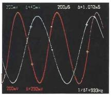
Another feature of the 5116 with the 5D10 is a direct readout of frequency or  $1/\Delta T$  (see display where  $1/\Delta T = 933$  Hz). This is one less step for you to get your measurement results.
