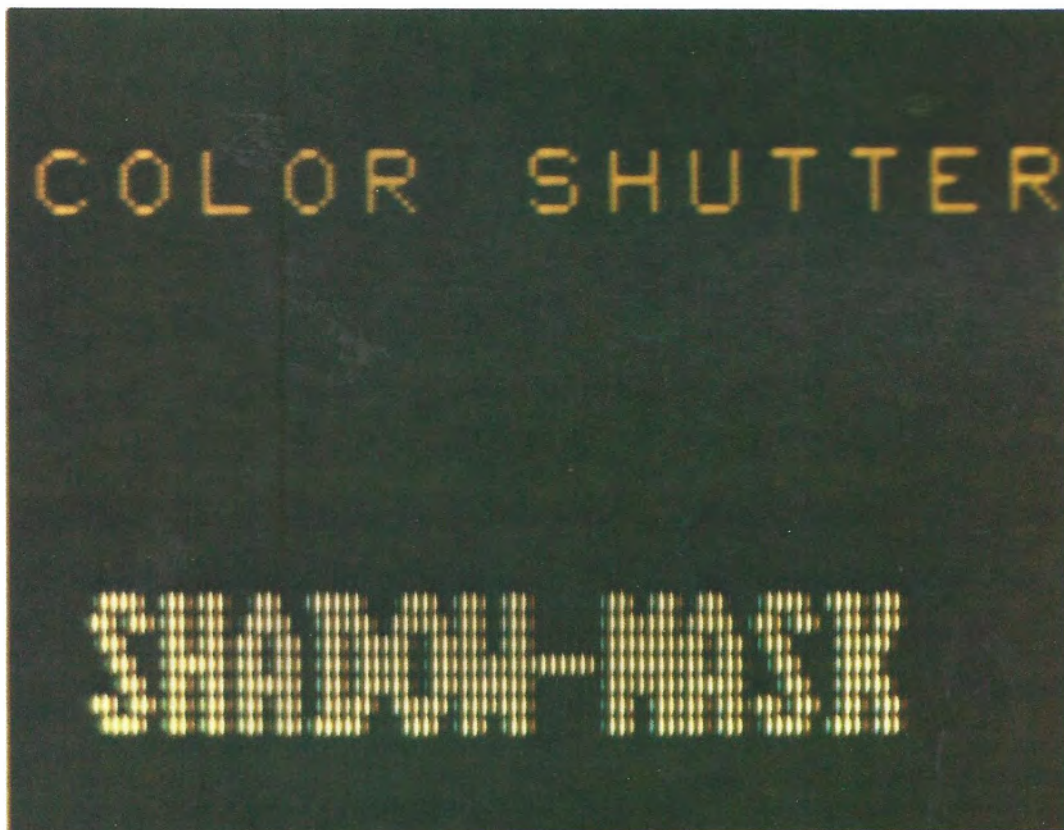
FIG. 1. Pictures taken from the screen at the same magnification from (a) a field-sequential display and (b) a shadow-mask display.
