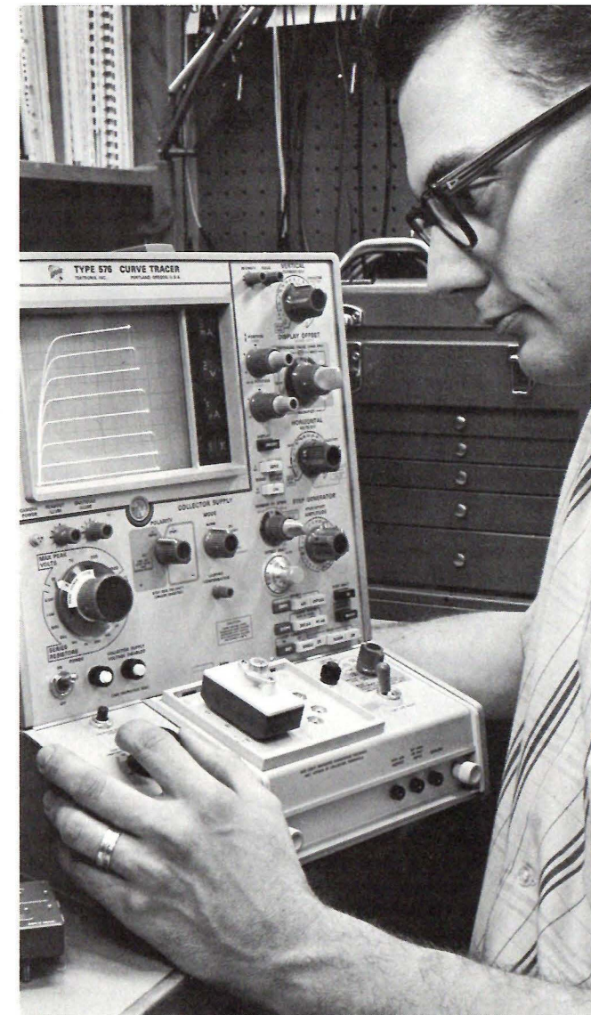
MANY NEW Tektronix-manufactured components made their first appearance in the Type 576 semiconductor curve-tracer.
