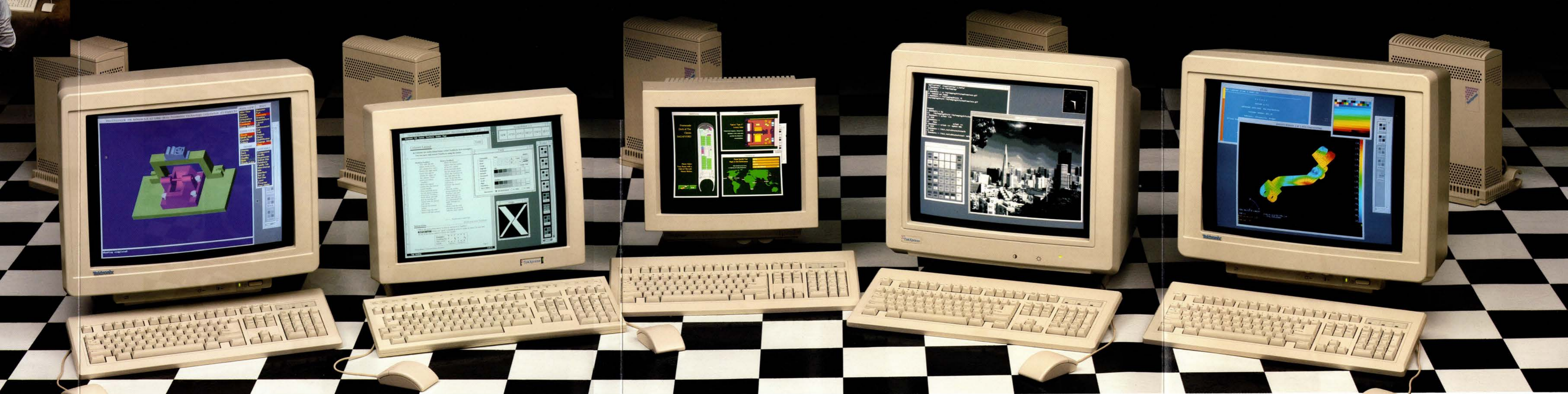
The TekXpress XP27. Providing 1152 x 900 resolution in a 19-inch color monitor, the XP27 is a popular choice for applications networked to Sun workstations, which feature identical pixel resolution. A 72 Hz refresh rate makes for easy viewing even over long stretches.
