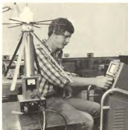
Bob Woolhiser using a Tektronix 7L12 Spectrum Analyzer to test for electromagnetic radio-frequency interference conducted from a Tek product (not in picture). The antennae in the foreground is used for radiated-emissions testing.
