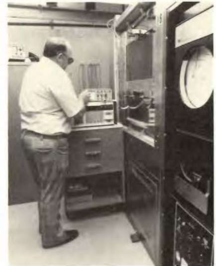
Humidity testing exposes a Tektronix product to a sequence of carefully controlled temperature and humidity conditions in a chamber. The chamber is to the right of Jim Smiley, who is adjusting a strip-chart recorder to log test conditions.
