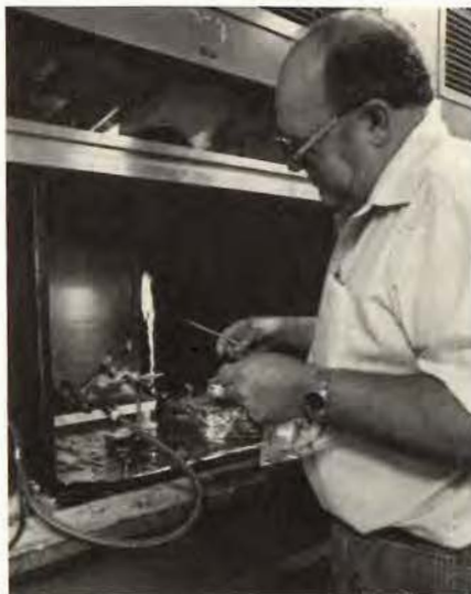
Jim Smiley is testing the flammability of a plastic.
