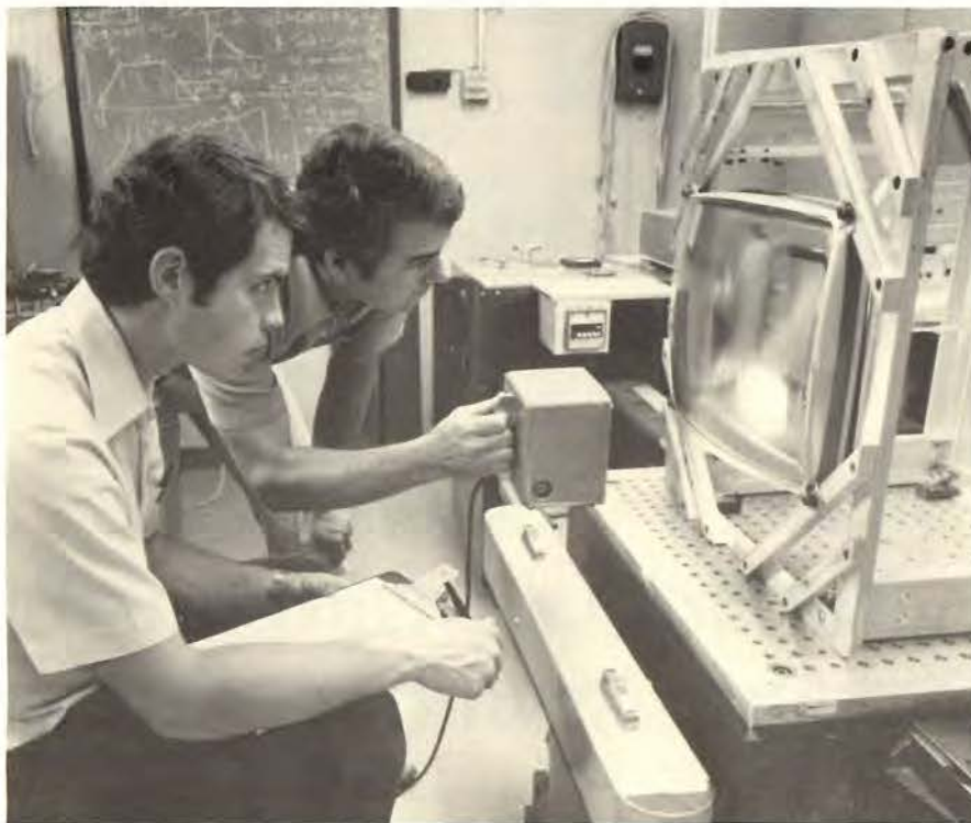
Joe Sanelle (left) and Tom Basta test a large Tek-made CRT for resonances on a shake table.
