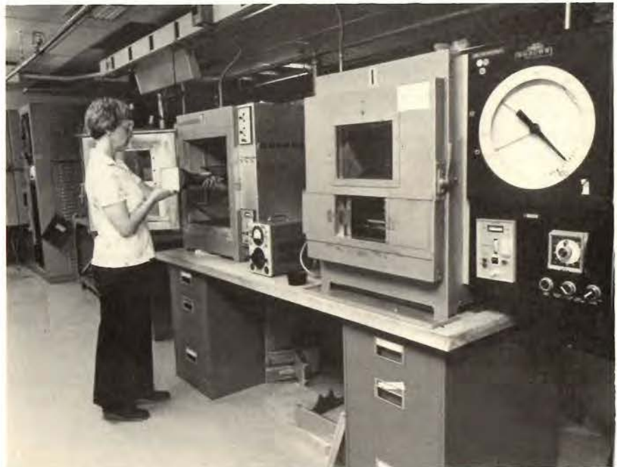
Jo Ann McCollister preparing a CRT for high- and low-temperature tests in a test chamber.
