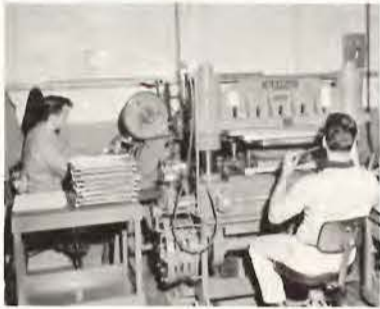
Gordon Bennett, forming the rounded corners on panels, and Douglas Dwight to the left operating the corner clipper which removes excess metal left by the punch.
