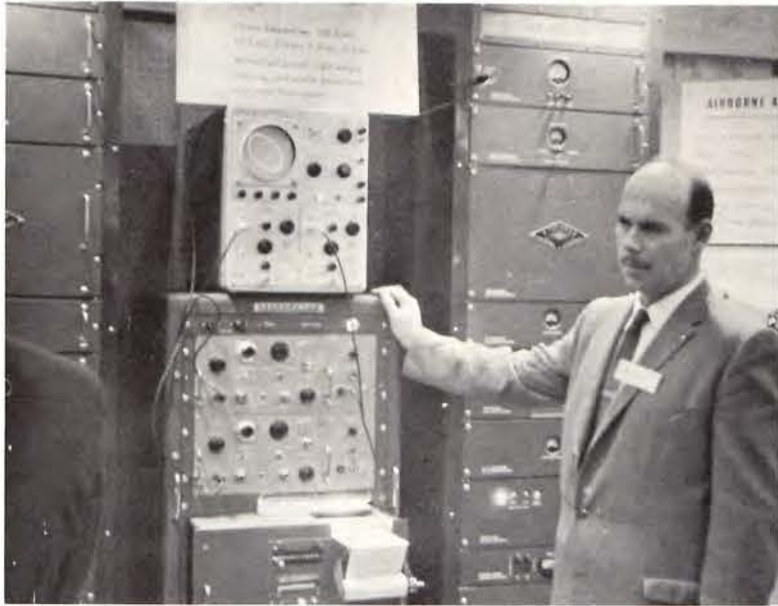
John Adams, field engineer from our Boston office checks on the performance of this scope which was used by National Company to indicate the accuracy of their Atomichron. The scope monitored the output of two of these atomic clocks to show any difference that might indicate any drift or inaccuracy. It turns out that the accuracy is one part in a billion or about equivalent to the loss or gain of 1/300 of a second second in a year. The Tek scope interprets the synchronous motion of the two clocks by the elliptical pattern on the face of the scope.
