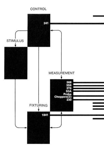
the system can repeat different tests (when less than 15) at different sets of pins, to a maximum of 150 tests. Fixtures may be customer supplied. A wide variety of fixture cards is available for the 1841 Fixture Drawer; these include cards for DTL, TTL, diode, and transistor devices. See page 27 for details.
