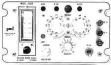
The 2005A Power Supply is manufactured by Power Designs, Inc., and is a precision supply mounted in a rack adapter that also permits adding a second supply at a later date. The supply features a digitally selected operating range from 0 to 20 V, 0 to 500 mA; accuracy is within 0.1-pct  $\pm$  1 mV; load and line regulation is better than 0.0005-pct or 100  $\mu$ V; noise and ripple are less than 100  $\mu$ V p-p, and stability is less than 100  $\mu$ V drift per 8 hours.
