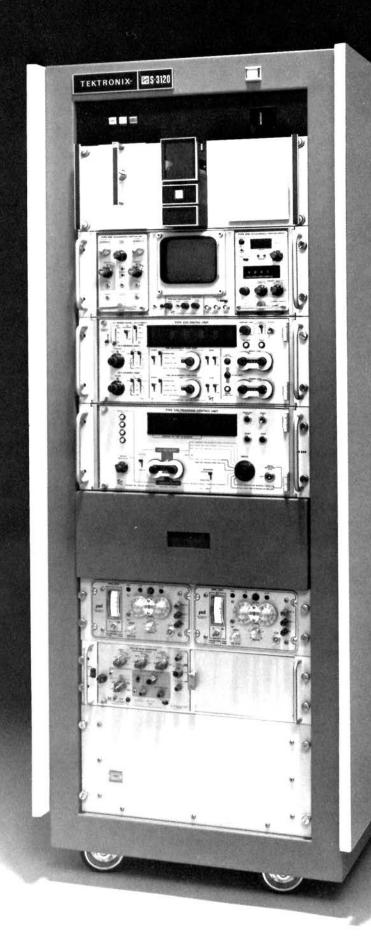
The S-3120 Automated Measurement System also uses the S-3101 measurement package, but linked with the R240 Program Control Unit and an eighttrack disc memory. The use of a disc memory permits a total of 1600 tests to be stored and then performed at up to 100 tests per second, giving this system an increased capability not only in versatility, but in capability for the number of measurements stored.
