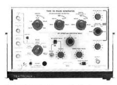
The R115 Pulse Generator features output connectors on the rear panel. The following functions may be set from the front panel: 10-ns to  $100-\mu$ s separate and variable rise times and fall times, 100-ns to 10-ms pulse periods, 50-ns to  $500-\mu$ s pulse delay or burst time, 50-ns to  $500-\mu$ s pulse width, +5-V to -5-V dc offset and up to  $\pm 10-V$  amplitude into 50 ohms.
