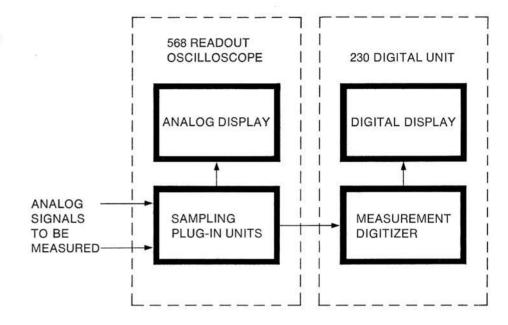
The 3100-Series automated measurement systems use a package consisting of a programmable readout oscilloscope (568), dual channel vertical sampling plug-ins (3S5/6), and delaying sweep time bases (3T5/6), plus a digital readout unit (230). (The primary function of the digital unit is to make digital measurements of sampled analog data.) Results are then compared with programmed limit values for automatic indication of whether the measurements are above, within, or below the predetermined limits.
