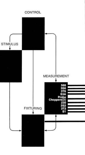
package to be externally programmed. In the 3S6 sampling unit, deflection factor, dc offset, and smoothing may be programmed. In the 3T6 sampling sweep unit, time per division and digital delay are programmable, and, since an automatic trigger circuit usable from dc to 100 MHz is included, no trigger programming is required.
