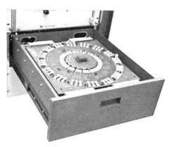
The 1840 is either rackmounted or mounted in a drawer. A Type A Load Board, furnished with the fixture, allows automatic testing of devices with up to 16 active pins. An optional Type B Load Board allows automatic testing of devices with up to 32 active pins. Inexpensive plug-on socket cards for each load board permit unique circuit configurations for each device tested. Devices with 16 pins or fewer usually require socket card change only when unique load circuits are used.
