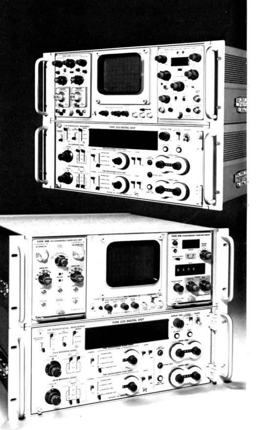
point, and polarity. Controls provide for upper and lower measurement limits. These limits function automatically for each digital reading and panel lights indicate whether results are above, below, or within limits. Thus, a measurement can be repeated many times, with the operator proceeding on the basis of limit indications rather than digital readings.
