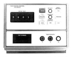
The standard Test Station Control Unit can be used with any test station, and provides system stop/start control, address of the test sequence, system status indicators, and test result indicators. This unit is small and portable, is equipped with a magnetic base, and may be located anywhere on the test station.
