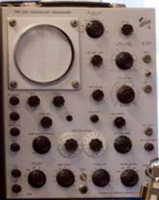
514D OSCILLOSCOPE The 514D had a bandwidth of 50 MHz and a sensitivity of 10 mV/cm. It was the first oscilloscope to have a built-in storage oscilloscope (BISO) section for recording waveforms.
